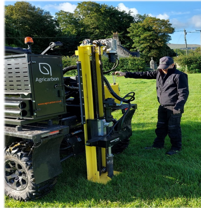
Soil Sampling to one metre deep
